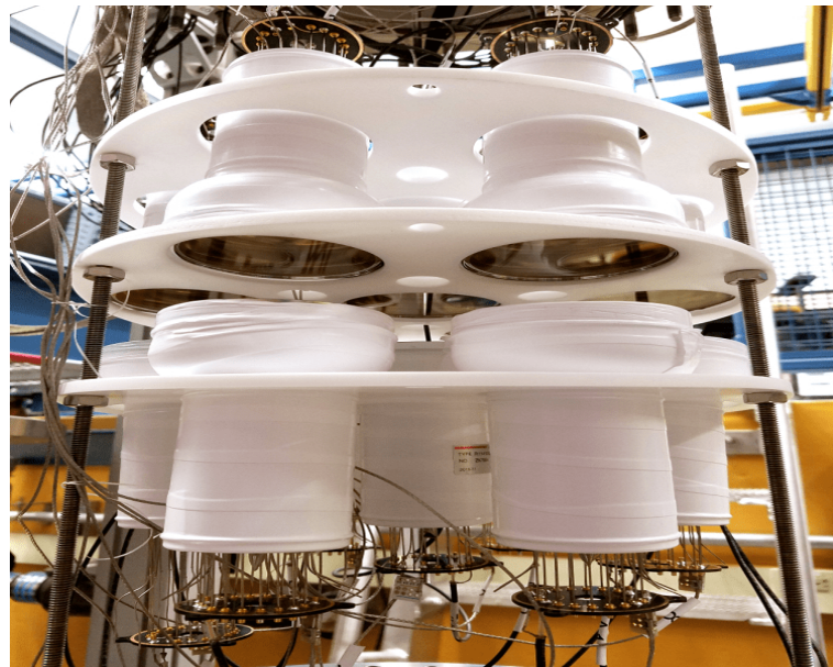
Figure 2.2: The Brown testing unit allows for 14 PMTs to be simultaneously tested in cryogenic temperature and pressure conditions (Credit: Brown University)
