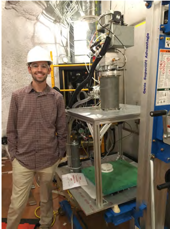
Figure 2.7: A picture of the author standing next to the D-D neutron generator in the Davis Cavern in the summer of 2016.
