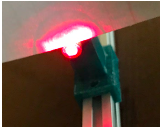
Figure 6.7: Reflection of the opposite mirror mount at the laser diode
