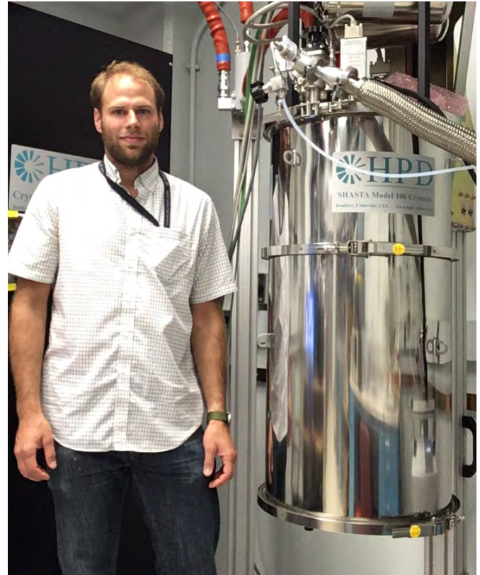
Nagler standing with the adiabatic demagnetization refrigerator used for sub-Kelvin PIXIE detector characterization
