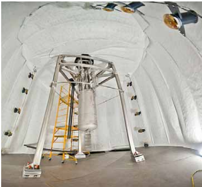
The Lux detector, hanging at the center of its 25 feet diameter water tank, which serves as a radiation shield and is itself instrumented as a Cherenkov light detector. The tank was filled with water in September 2012, one of the few last steps needed toward getting ready to turn the experiment on for dark matter hunting.
