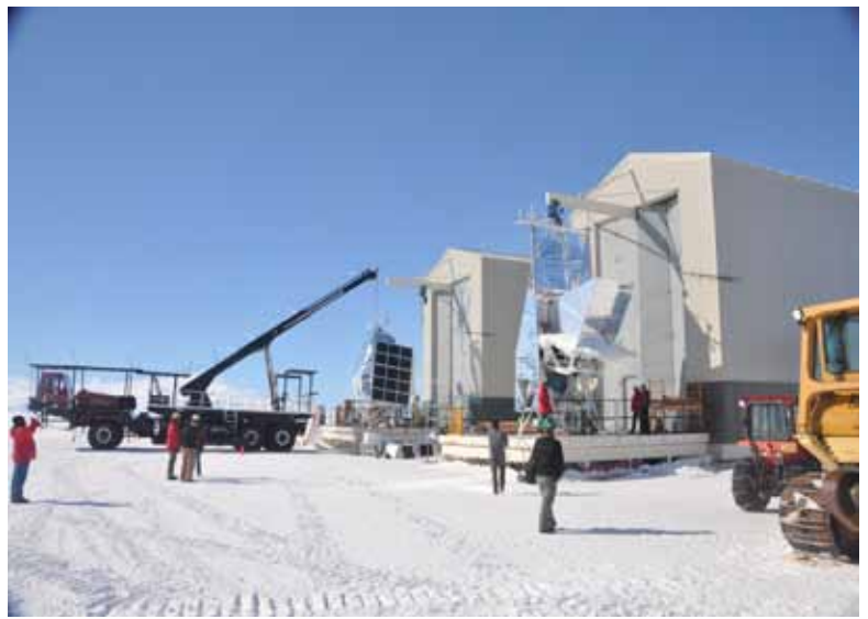
A rare site, BLAST-Pol (left) and EBEX (right) outside for testing at the same time. The launch vehicle (aka The Boss), is attached to BLAST-Pol in preparation for testing.
