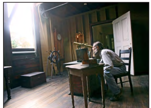
Michael Umbricht, a Ladd staff member, sits in the recently restored Transit Room gazing through a portable telescope, which once was used to make accurate time measurements through observations of the stars
