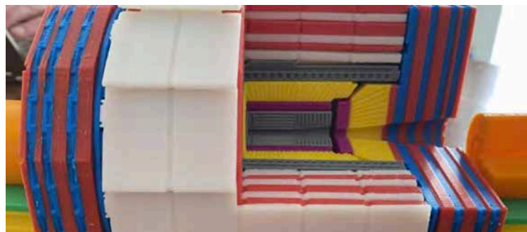
Prof. Heintz's 3D printout of a detector. The gray component, the tracker, is the piece that Prof. Heintz and his students are building for the Large Hadron Collider at CERN. Photo: Valerie DeLaCámara/Brown University
