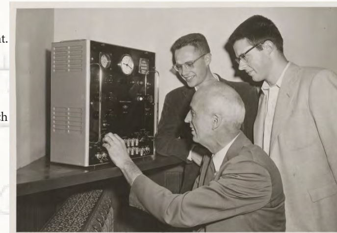
Professor Smiley demonstrating a quartz frequency standard to students at Ladd Observatory.
