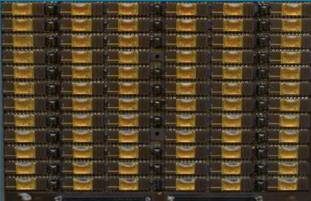
A close up view of the semiconductor memory chips in the computer. Courtesy: Dave Fischer
