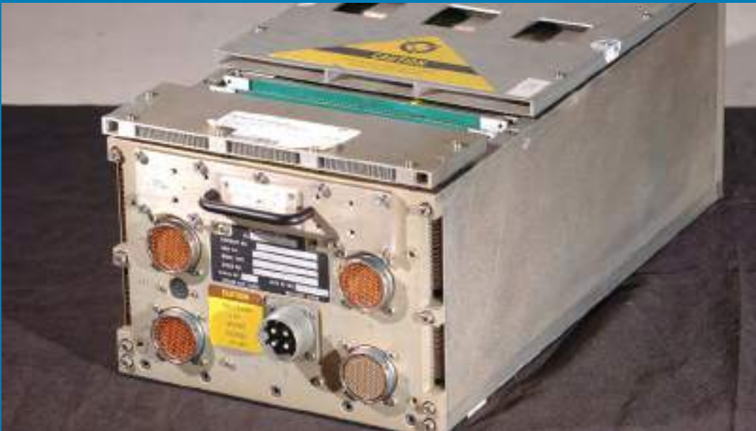
A second-generation space shuttle computer with the top cover removed. Courtesy: Dave Fischer
