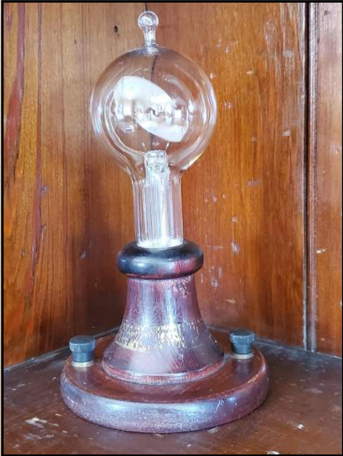
A replica of Edison's 1879 carbon filament light bulb. Made in 1929 by General Electric Co. for the 50th anniversary.
