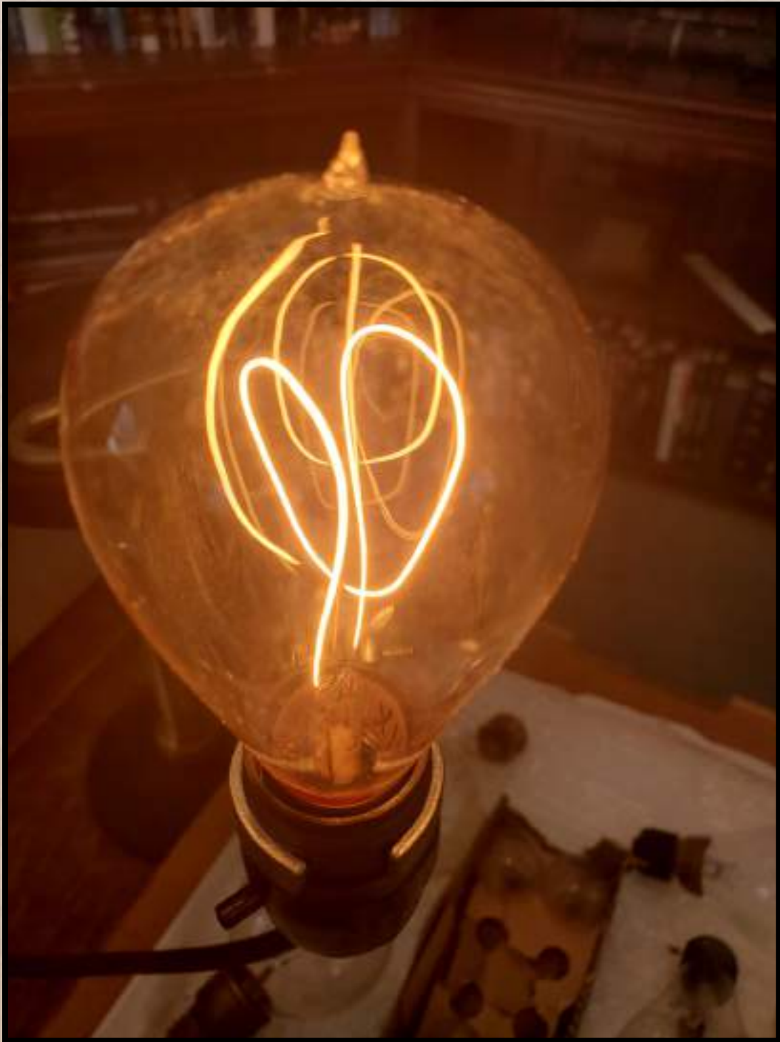
An early carbon filament light bulb. It was likely made before 1915. It uses about 30 watts.
