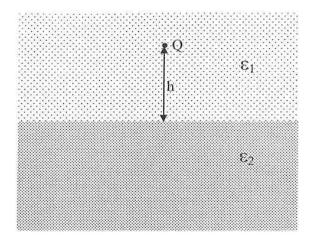
A point charge Q is embedded in a semi-infinite medium with dielectric constant  $\epsilon_1$ , at a distance h from an interface with another semi-infinite medium, characterized by the dielectric constant  $\epsilon_2$ .
