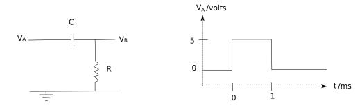
Consider the circuit in the figure composed of a resistor and a capacitor, with  $R = 1k\Omega$  and  $C = 1\mu F$ .
